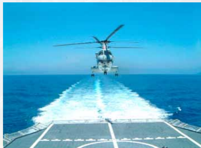
Incat vessel Helo Deck, Kevlar reinforced epoxy anti-slip coating
